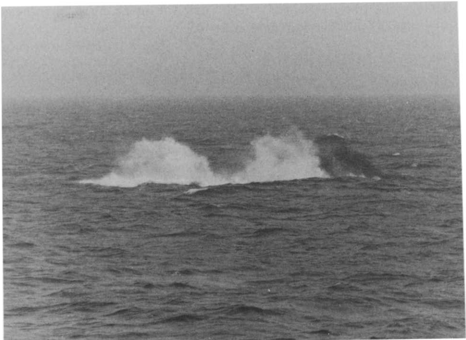
Fig. 5. Gas bubble 2.2 s after the detonation.
